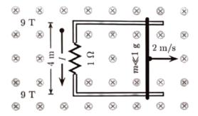
Calculate the applied force required to move the bar to the right at a constant speed of 2 m/s. Assume the bar and rails have negligible resistance and friction. Neglect the mass of the bar. Answer in units of N.
